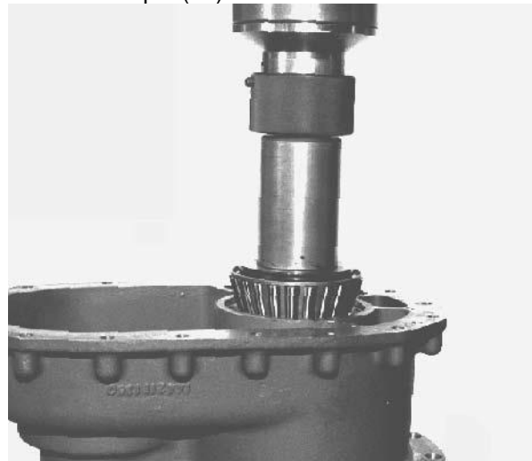
Picture 9. Pinion bearing installation and adjustment.
