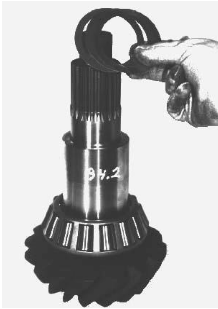
Picture 8. Pinion with inner bearing cone installed.
