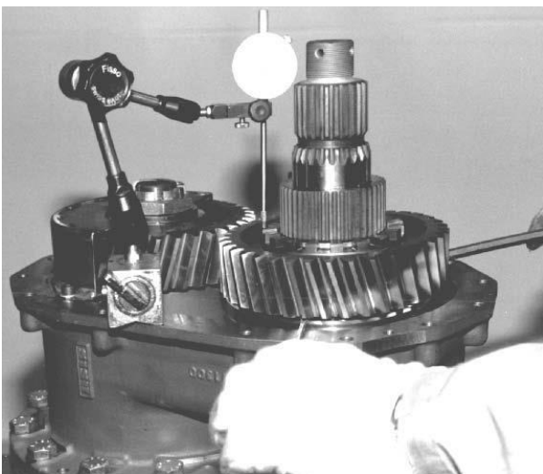
Picture 18. Clearance check with a dial indicator.
