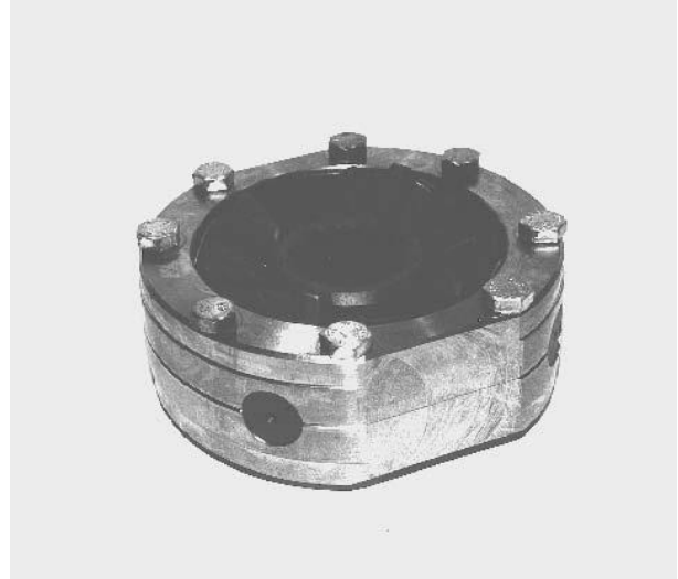
Picture 4. Inter-axle differential assembly.
