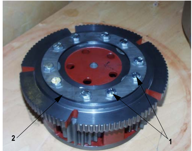
Picture 4 Planetary gear removed
